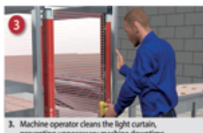
3. Machine operator cleans the light curtain, preventing unnecessary machine downtime.
